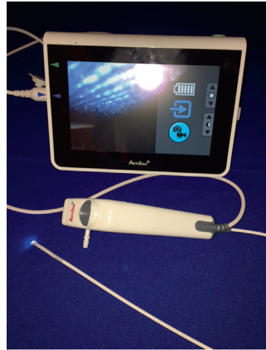
Fig. 1.19. The Ambu aScope is a new, fully disposable video flexible bronchoscope with an integrated suction port and working channel for suctioning and instillation of local anesthetic. Airway images are viewed via a reusable digital display. (Courtesy Calvin A. Brown III, MD.)
