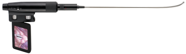
Fig. 1.16. The Clarus Video System incorporates a curved stylet containing a CMOS chip video camera surrounding by a malleable but rigid protective metal sheath. Images are displayed on a video screen attached to the handle. The screen can swivel for optimal viewing as the stylet is inserted into the mouth. (Courtesy Clarus Medical, Minneapolis.)
